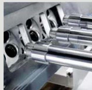
Controlled pressing of valve seat rings with electric press spindles
