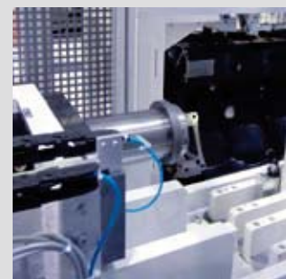
Force fit sealing parts and leak-test
